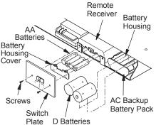
Figure 31 - Installing Receiver Batteries (Included)
